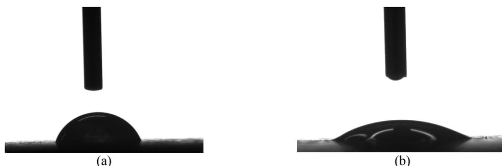
Fig. 3 Contact angle measurements for (a) before and (b) after irradiation with the UV lamp for 8 h
